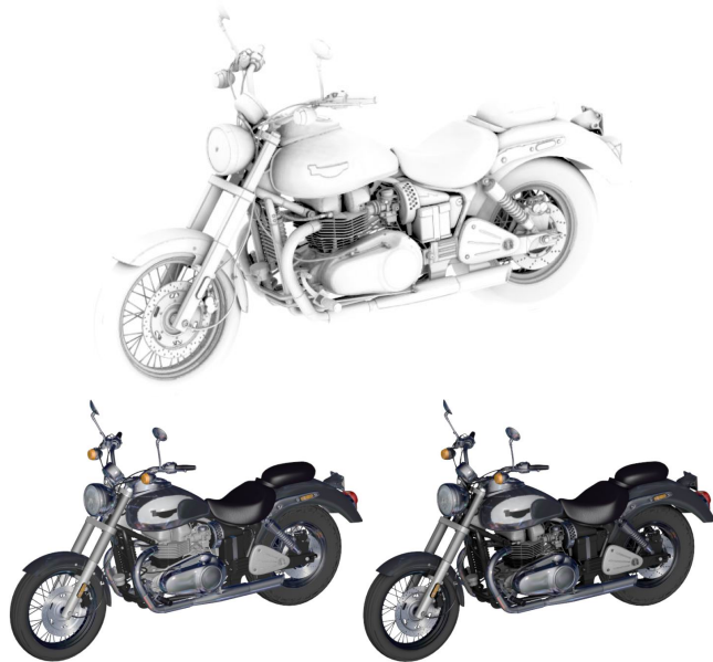
Figure 6: Top: Ambient occlusion map applied to white surface. Bottom: Final frame without (left) and with (right) ambient occlusion texturing.
